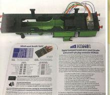
The next part of the puzzle is finding space for the Zimo MX648R sound decoder and as we have already seen, decoder space is limited. The Zimo decoder leaflet opens out and has a dear diagram showing the earth (ground) terminal on the decoder to which the black 'stay alive' wire then fits, and the blue wire goes to the terminal where the decoder's own blue wire originally went, or join it directly to the blue wire if you decided to leave it on.
