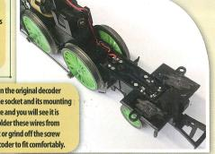
Preparing the decoder for hardwiring is the next stage and this could be the trickiest job. It is best to unsolder the unwanted cables from the decoder and then fit the new 'stay alive' wires to it. The connection points are accessible after trimming the sides of heatshrink covering enough to fold it back: it can be put back and secured with tape later to restore the insulation.
