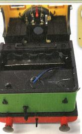
You'll be pleased to learn that the only metalwork alteration on the body casting is to drill out one of the water filler mounting holes a little bigger for the 'stay alive' wires to go through.
