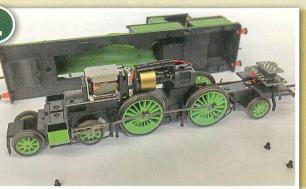
The Oxford Rail Adams '0415' 4-4-2T is an easy model to open with two screws at the back and one at the front. The leading screw is accessed through a hole in the front bogie. The body lifts off without any other parts joining it to the chassis - no hidden pipes or wires to catch out the unwary.
