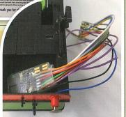
This picture shows the connections and the 'stay alive' wires fitted. The 'stay alive' wires will be coming through the bunker casting. Remove the wires not needed - brown, green, blue, white and yellow - although you could cut them neatly and secure them tidily away if you prefer. The advantage of removing them completely is that it saves space and reduces the possibility of short circuits against the metal chassis bodyshell.
