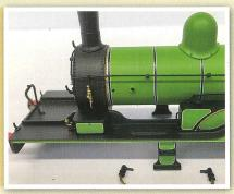
The key thing to look for now is that the speaker wires align with the groove in the chassis for the existing wires under the cab floor. Note the purple speaker wires on the body already positioned to line up with the red and black wires in the locomotive chassis. Lay the body on its back and place the chassis into it checking all wires are tucked
