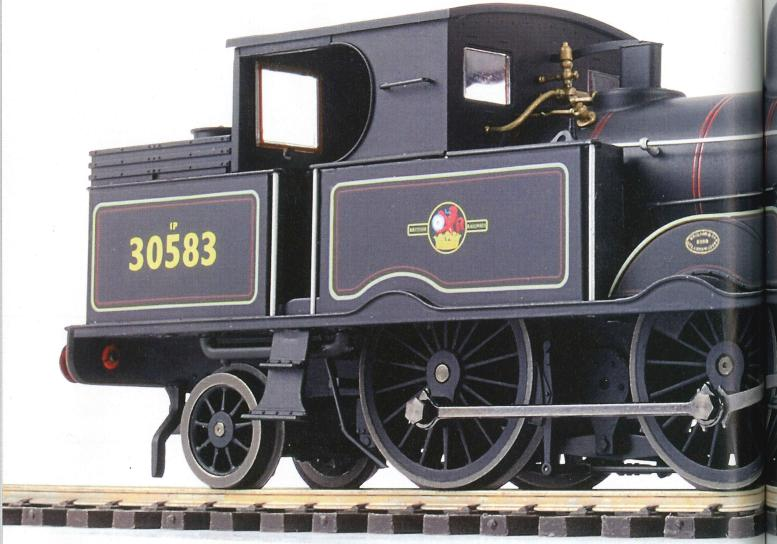
HIS ADAMS 'RADIAL TANK' was Oxford Rail's first 'OO' gauge ready-to-run locomotive (HM103). Oxford made modifications to the chassis design after the first version modelling 30583 in BR livery was produced, allowing the front bogie more vertical movement, and it has proved to be a reliable and capable locomotive.
